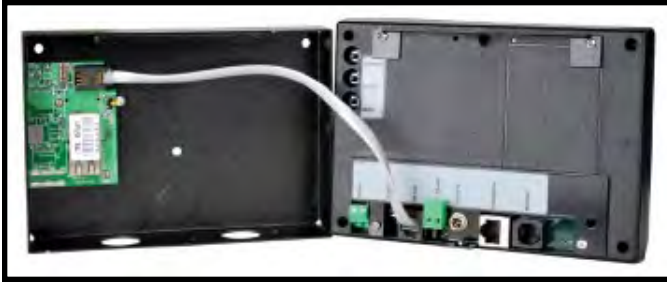
Figure 3. Connecting the Ethernet Board to the Smart Clock
